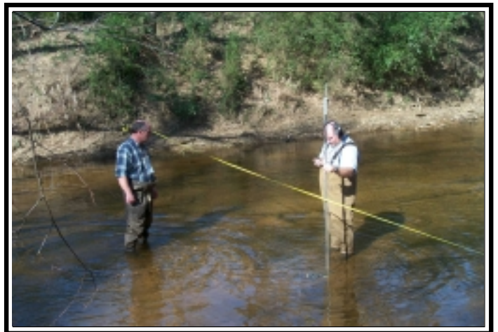
Charles Babb, NRCS Left and Keith Butler, Town of Chesterfield Right, taking velocity measurements in Thompson Creek.
